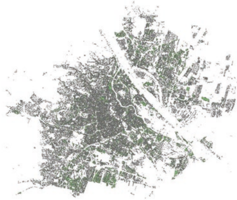
Fig. 4 Flat roofs identification and mapping with ARCGIS (Source: Dang 2016)
