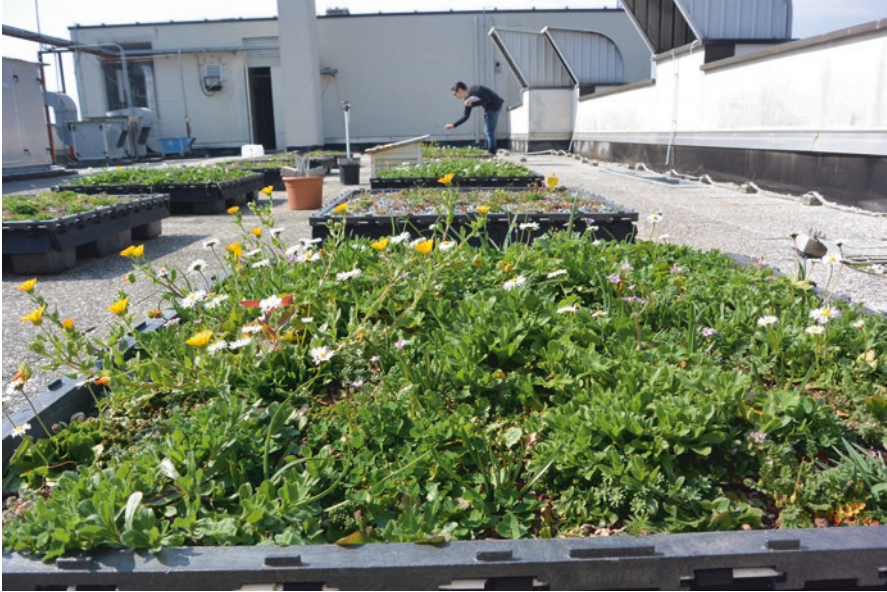
Fig. 3 Trials on a green roof with native herbaceous species to improve the urban biodiversity (Photo Francesca Bretzel)
